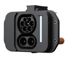
Standard:IEC 62196-1-2022 IEC 62196-2-2022 IEC 62196-3-2022 Rated current: DC 80A/125A/200A/250A AC 16A/32A Rated voltage: DC 750V DC/1000V DC AC 250V AC/480V AC Operating temperature:-30°C  $\sim$  +50°C IP degree: Covered IP54/ Inside IP67/ Mated with Plug IP55 Insulation resistance:>1000M $\Omega$ Mechanical life: > 10000 times Flame retardant rating: UL94-V0 Terminal temperature rise: < 50K Environmengtal requirement: RoHS compliant
